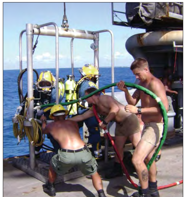
Putting divers down to rig onto a DTON using 1 1/4 Wire.
