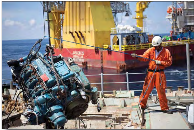
SMIT salvage contractor guiding main engine as it is being lifted from the Ex-USS Guardian funnel section.
