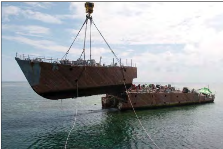
Ex-USS Guardian bow section lift - 314 tons.
