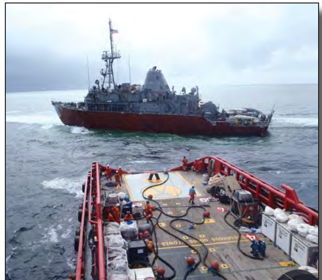
Hydrocarbons and hazardous materials being pumped from Ex-USS Guardian to the VOS Apollo.
